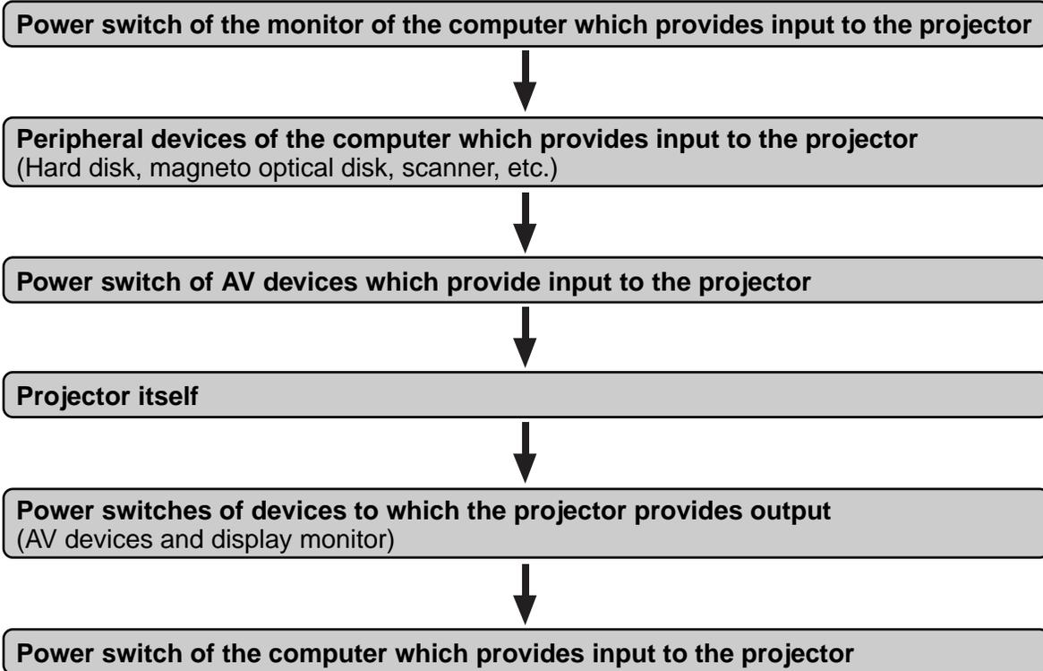
\* When turning off the power switches, do so in the reverse order.
